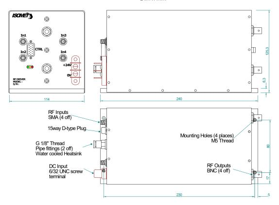
Control signals on 15 pin high density 'D' type (compatible with iMS4-x synthesizers, J5 output):
